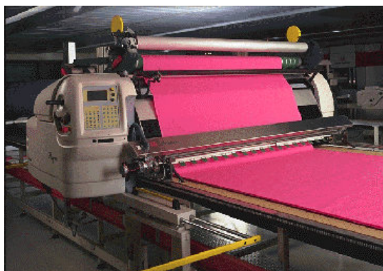
(E) Fabric Laying in Cutting Machines
