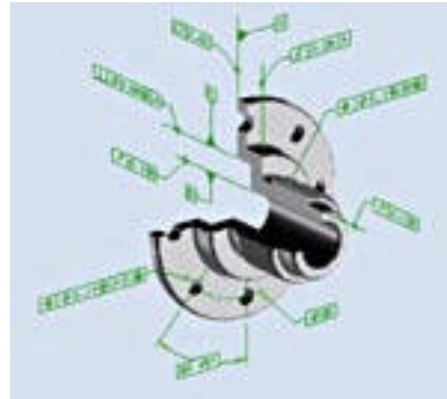
(F) Geometric tolerances on a solid model.
