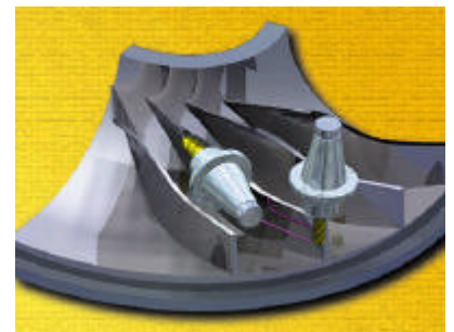
(F) Multi axis and multi spindle milling
